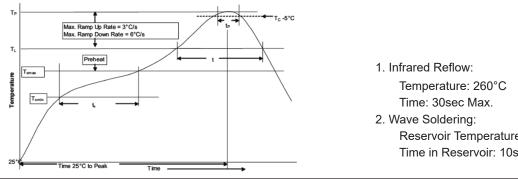
Newark.com/multicomp-pro Farnell.com/multicomp-pro sg.element14.com/b/multicomp-pro Reservoir Temperature: 260°C Time in Reservoir: 10sec Max.
