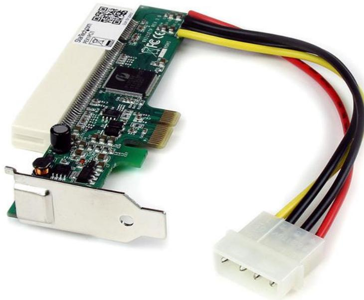
This PCIe to PCI Adapter Card lets you use low profile PCI expansion cards in a server or desktop motherboard PCI Express slot. Compliant with PCI Express Specification 1.0a and PCI Specification 2.2, the adapter card connects through a PCIe 1x slot to provide a low profile PCI slot in its place. A spare full size bracket for PCI Express card is also included for use in larger desktop or server PCI Express slots.
