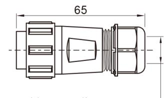
Cable outer diameter range: I: 4.5-7mm II: 7-12mm
