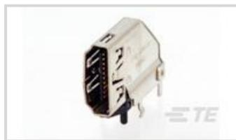
Connector & Housing Type: **Receptacle**Connector Profile: **Standard**Number of Ports: **1**PCB Mount Location: **Top**PCB Mount Orientation: **Perpendicular Right Angle**
