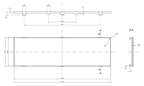
All dimensions are given within +/-0,5mm tolerance
