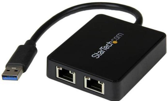
The USB32000SPT USB 3.0 to Dual Port Gigabit Ethernet Adapter lets you add two Gigabit Ethernet ports to your laptop or Ultrabook™ computer through a single USB 3.0 port, and features an integrated USB 3.0 pass-through port that keeps your USB port available for use with external storage or other peripherals. Each RJ45 port supports 10/100/1000 Mbps Ethernet and is fully compatible with IEEE 802.3i/u/ab standards.
