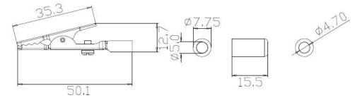
CLIP: STEEL, NICKEL PLATED BODT: ABS, RED/BLACK UNIT: MM
