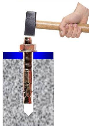
Insert assembled anchor through fixture into concrete
