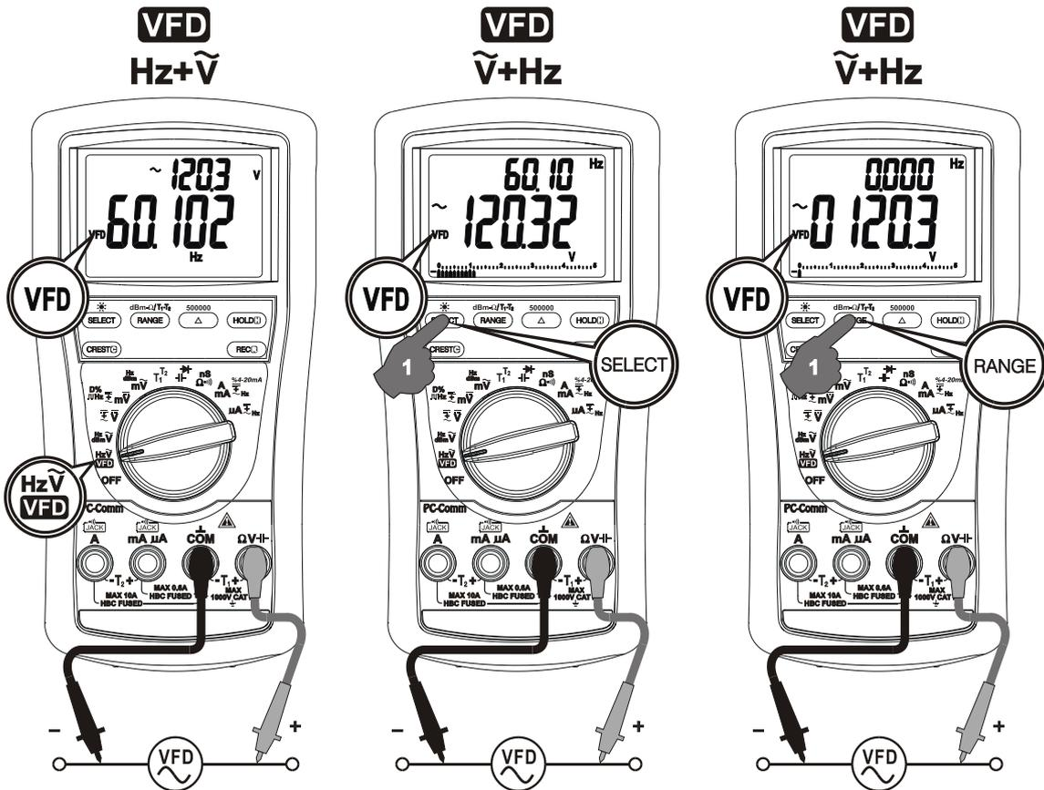
Note: Hz Input sensitivity varies automatically with voltage (current function alike) range
