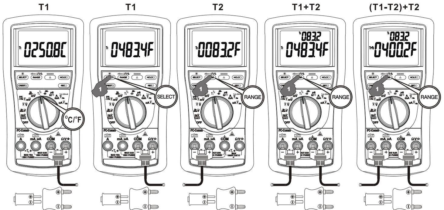
Note: Be sure to insert the banana plug type-K temperature bead probe Bkp60 with
