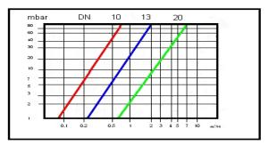
Therefore pressure drop (mbar) can be calculated for any given hose assembly adding P1 and P2.
