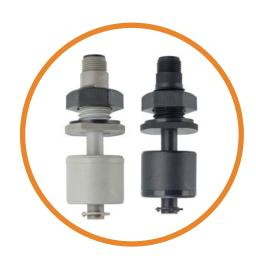
The RSF150 series are compact vertically mounted devices with a single switch point. Mounting is either from the top or bottom of a tank from the inside, so requires access to the inside of the tank.
