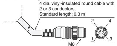
\* The Emitter cable has two conductors and the Receiver cable has three conductors.
