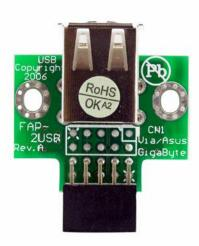
This USB A to USB Motherboard 4-Pin Header plugs directly into a motherboard USB header, providing two standard USB A female ports.
