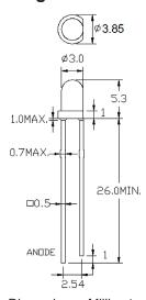
Dimensions : Millimetres Tolerance: 0.25mm
