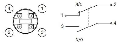
The switch is not polarity sensitive
