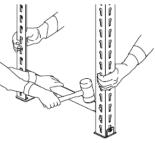
Locate top short beam, position at highest shelf position required.a
