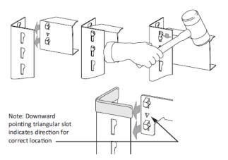
Locate base short beam, for the lowest shelf position, within 200mm of the floor (if exceeded, floor fixing is required).
