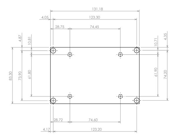
Dashed line shows outline of the mounting boss under PCB board Recommended mounting holes diameter ø3,5mm
