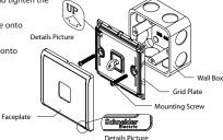
Insert a screwdriver into the clip lock, and twist the screwdriver to remove the faceplate.
