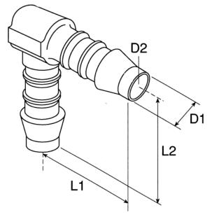
D1: Joiner Outer Diameter D2: Joiner Inner Diameter L1: Length
