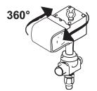
5. Press firmly to ensure coil is secured.
