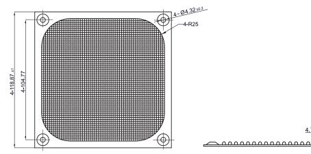
Dimensions : Millimetres General Tolerance Unless Noted: ±0.5mm
