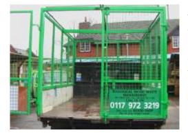
The rear of the truck should have twin gates with strong spring catches on both top and bottom to ensure there is no risk of the doors opening unexpectedly. It should be possible to secure the doors flat against the cage sides, although the vehicle should never be driven with the cage doors open.
