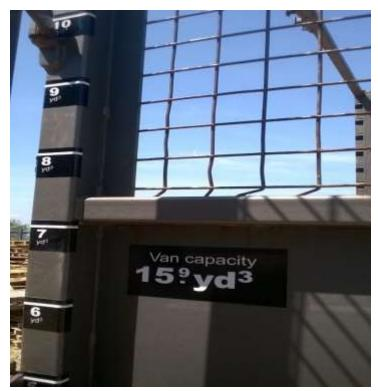
To help evaluate the load size fairly and efficiently, the vehicle should have the capacity of the cage signwritten on it. In addition, clearly visible "proportion full" marks should be placed up both sides of the cage.
