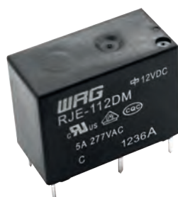
RJE Series Power Relay – 10A Dimensions: 19.8×9.9×15.2 mm Operating temperature: -40° +105°
