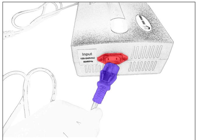
***Plug the Separate Cable into the Charger***
