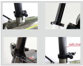
The minimum insertion mark of seat post must be under the seat post clip.
