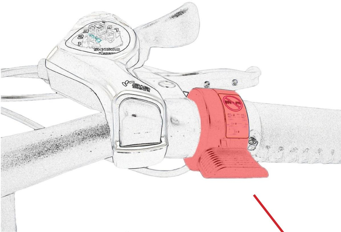
Gently pushing the throttle lever downwards to accelerate.
