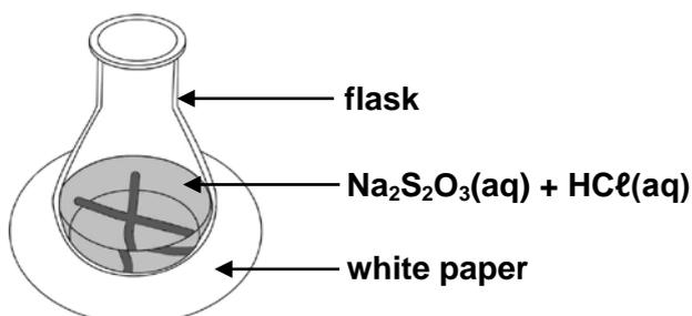
They measure the time it takes for the cross to become invisible. The experiment is repeated with the temperature of the mixture at 40 °C, 50 °C and 60 °C respectively.
