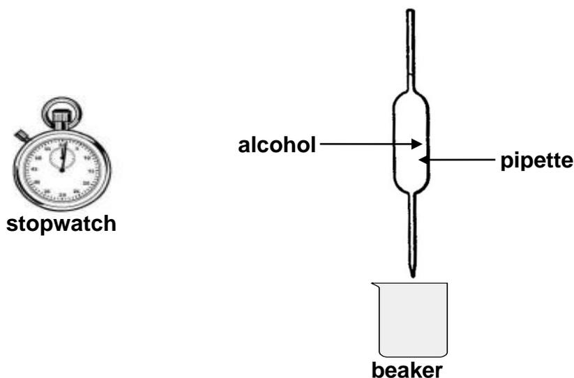
The learners use the stopwatch to measure the time it takes a **FIXED VOLUME** of each of the alcohols to flow from the pipette. They record this flow time, which is an indication of the viscosity of each alcohol, as given in the table below.
