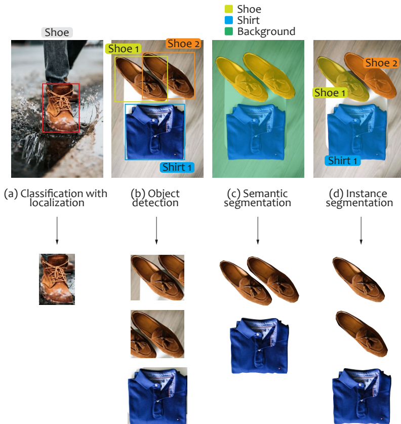
Figure R5.17: The four main problem formulations related to the localization task.
