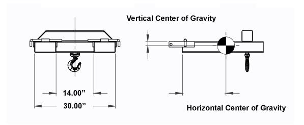
Model = MFSH-6 Empty Weight = 137 lbs Vertical Center of Gravity = 1.35" Horizontal Center of Gravity = 15.98"
