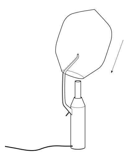
Carefully slide the glass shade down over the length of the arm until it reaches the support arm (\*)
