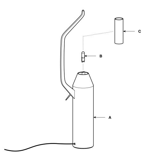
**4.** With one person holding the base steady, carefully lift the glass shade over the top of the arm of the base at an angle, as shown in the diagram.
