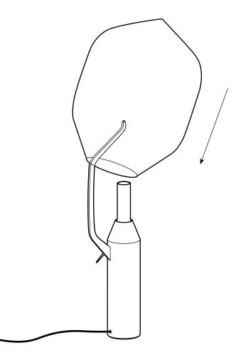
5. Carefully slide the glass shade down over the length of the arm until it reaches the support arm (\*)
