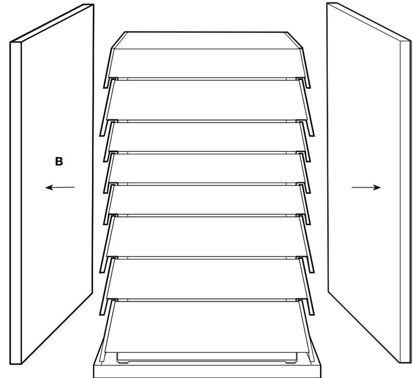
3. 2 people at the base and 1 supporting the top of the piece to prevent tipping. Carefully lift from under the bottom white drawer panels (C). The remaining person should quickly remove the base of the crate from underneath (D). **WARNING! DO NOT** lift from the side coloured panels (E). **WARNING! HEAVY ITEM**, there is a risk of injury if handled incorrectly.
