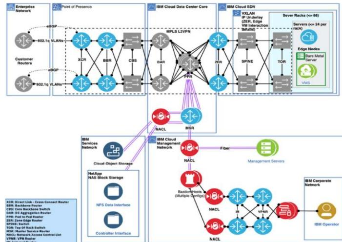
The logical network topology is shown mapping the data flow between components and provides a visual depiction of the system network components that constitute IBM Cloud VPC.
