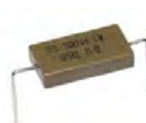
Ceramic encapsulation (selfprotected)
