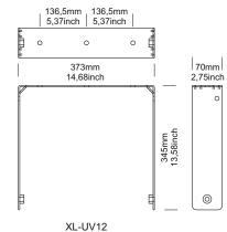
Wall metal bracket to mount in vertical position
