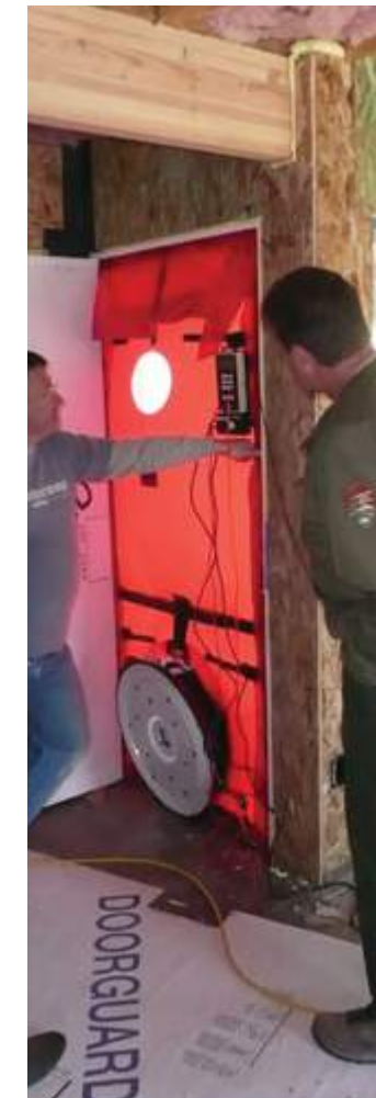
Blower door tests done before drywall is installed helps builders find and fix leaks.
