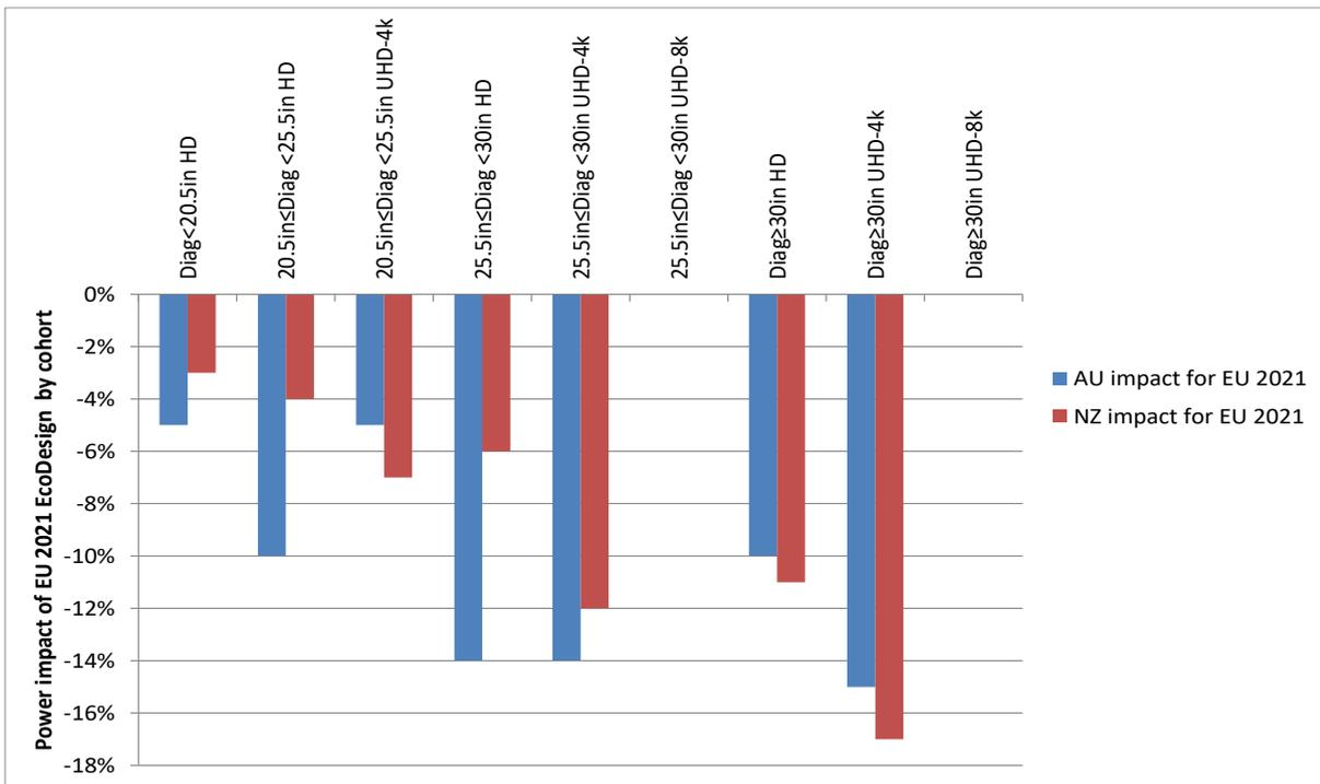
**Figure 35: Expected change in on-mode power of current computer monitors from EU 2021 MEPS**
