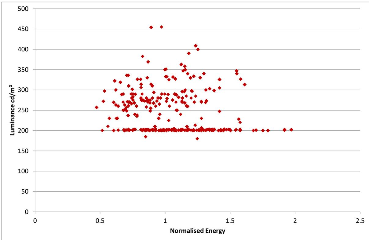
**Figure 61: Normalised energy versus brightest screen luminance for computer monitors sold in 2018-2020, Australia**
