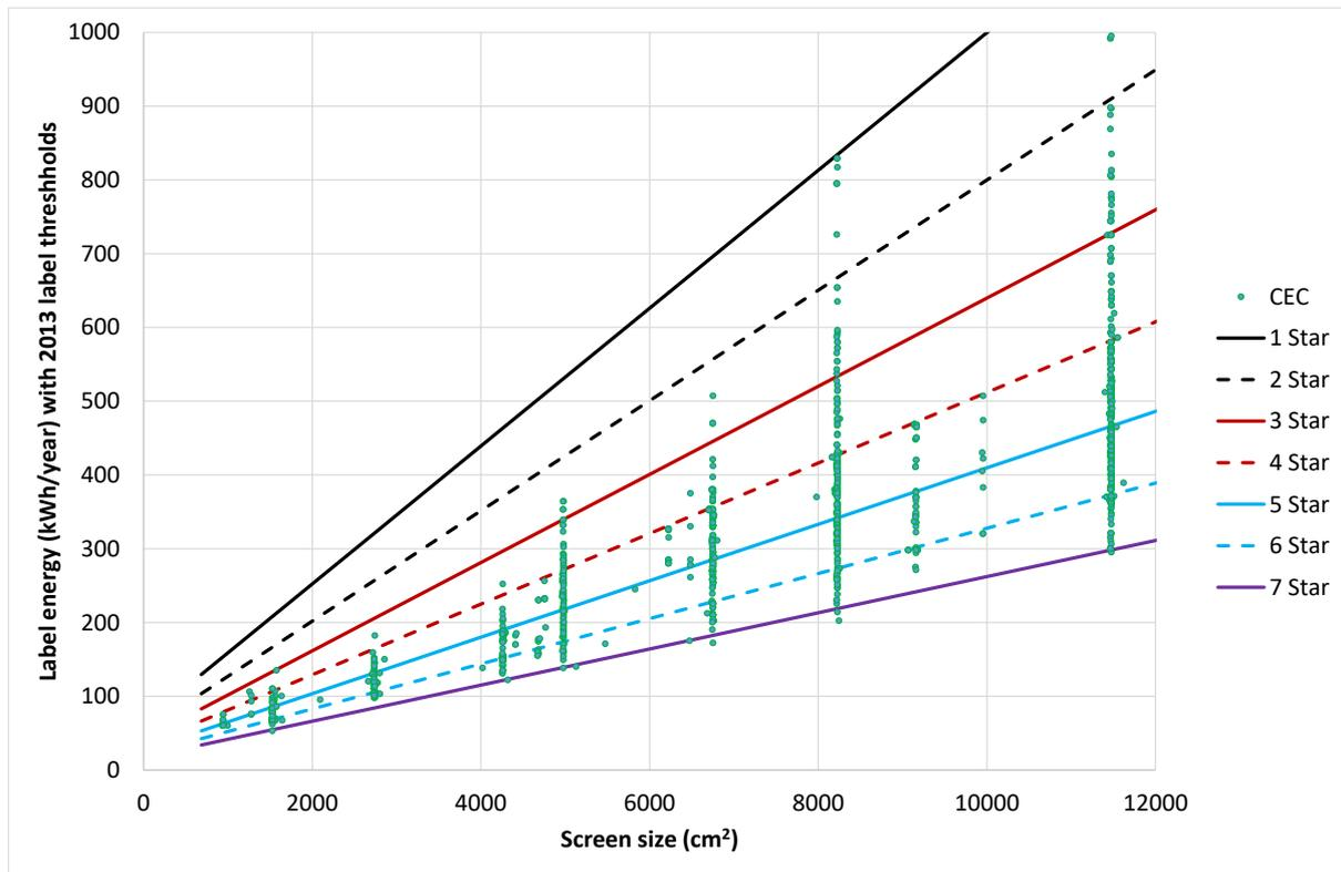
**Figure 12: Screen size and energy consumption of televisions registered in 2020 to 2022**
