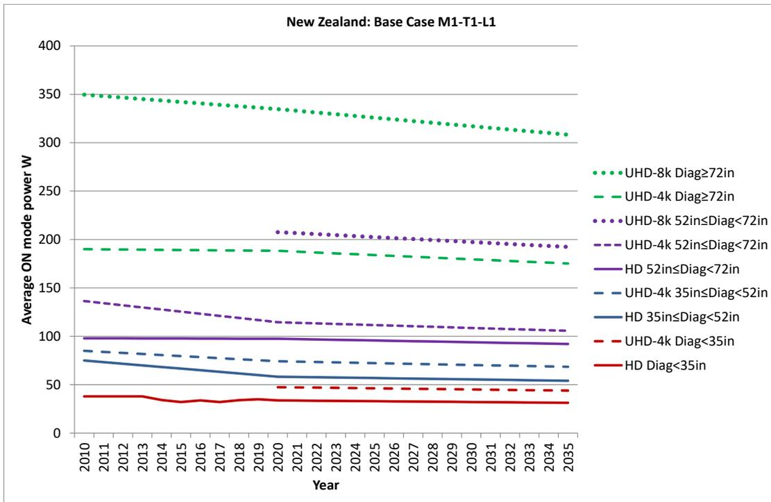
**Figure 14: Historical and projected on-mode power for televisions by size range and resolution, New Zealand. Sales weighted data to 2021, projections at -0.5% per annum to 2035. Average power within each size range will be increasing as the share of higher resolution models increases over time.**
