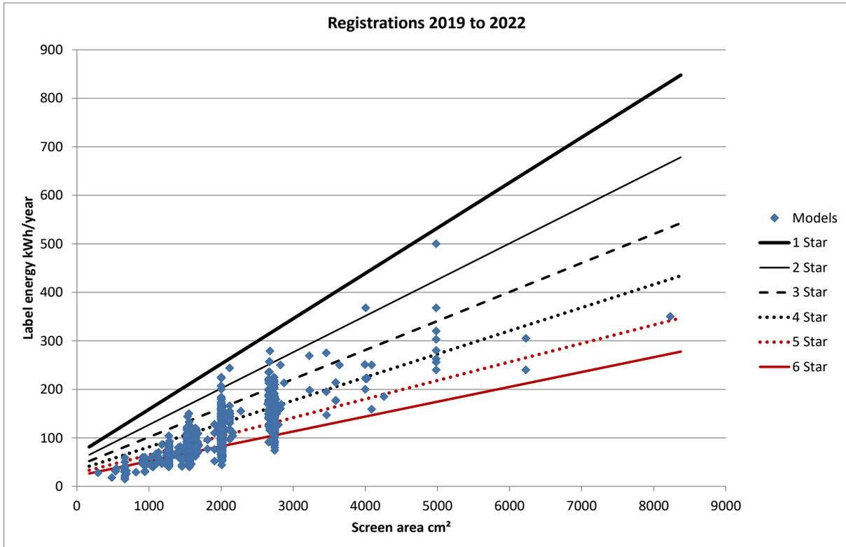
**Figure 28: Current computer monitor star rating bands with products registered 2019 to 2022**
