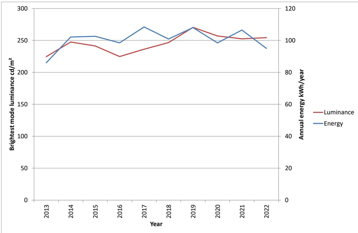
**Figure 56: Trends in energy and brightest mode luminance for computer monitors from GEMS registration data**
