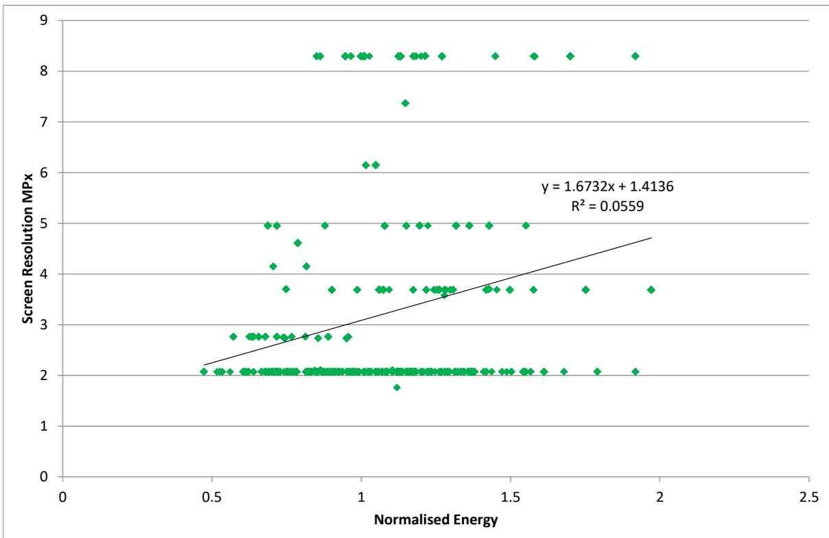
**Figure 62: Normalised energy versus screen resolution for computer monitors sold in 2018-2020, Australia**
