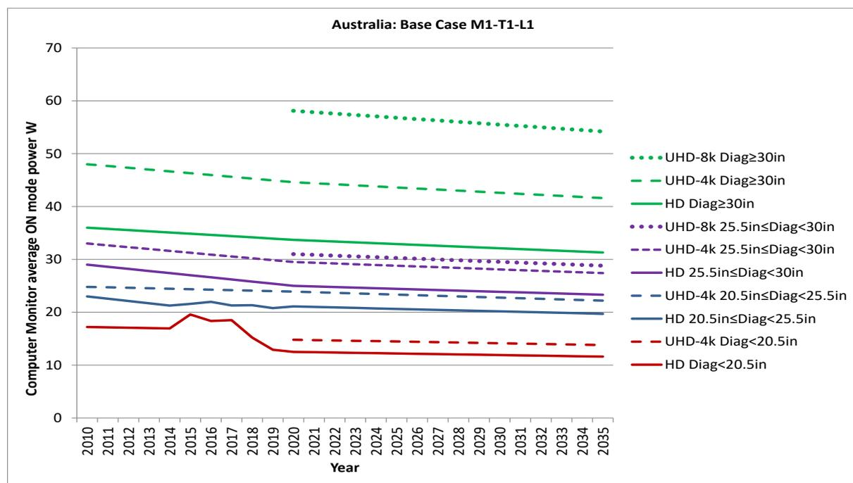
**Figure 31: Historical and projected base case on-mode power for computer monitors by size range and resolution, Australia**
