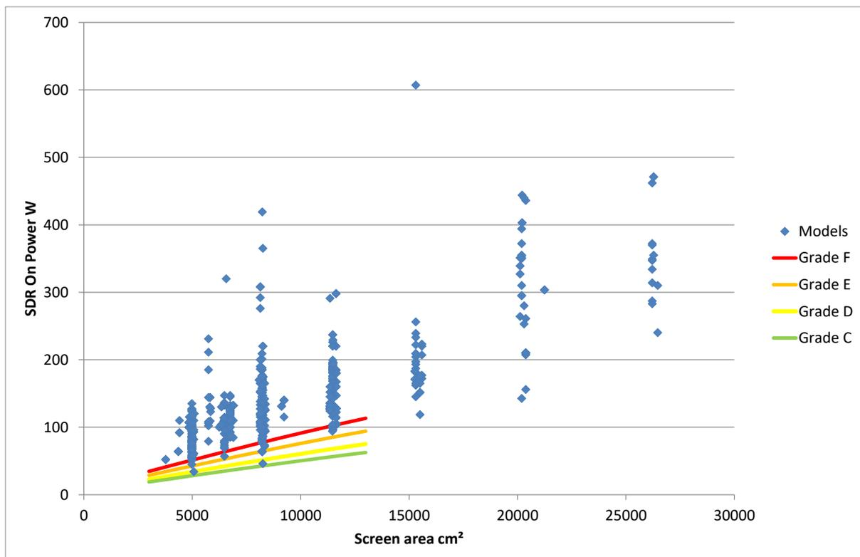
**Figure 38: Distribution of signage display models from the EPREL database – on-mode power for Standard Dynamic Range (SDR)**
