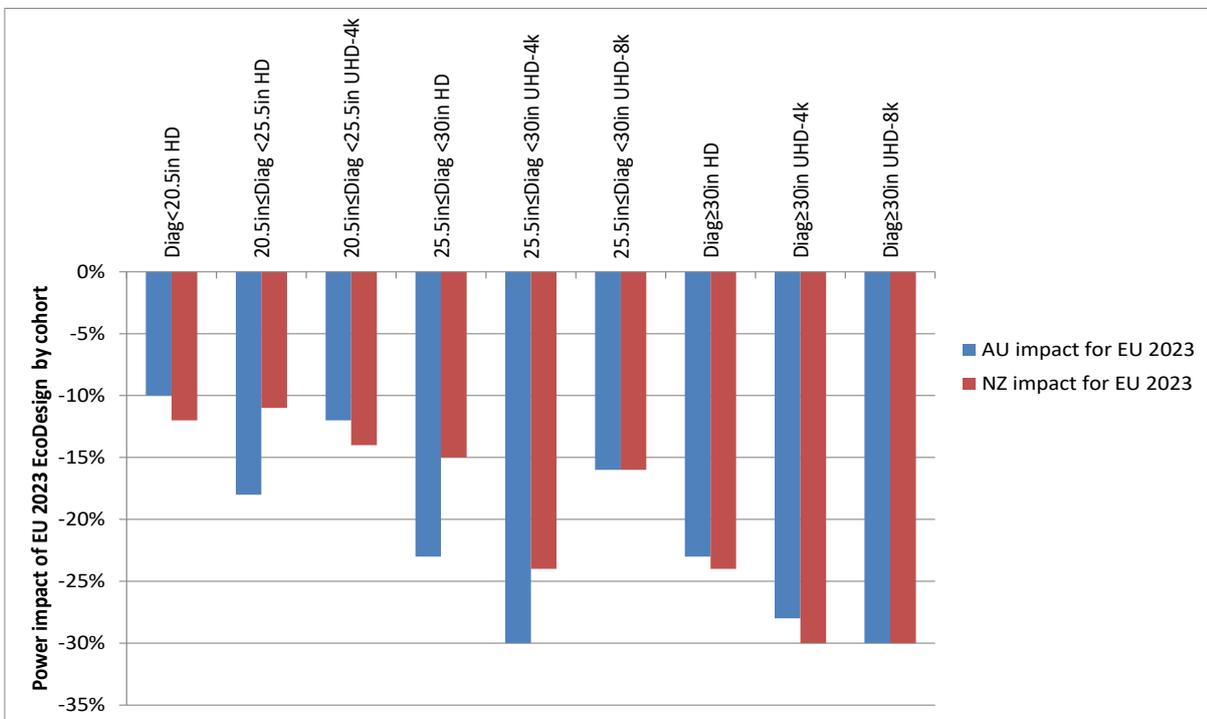
**Figure 36: Expected change in on-mode power of current computer monitors from EU 2023 MEPS**
