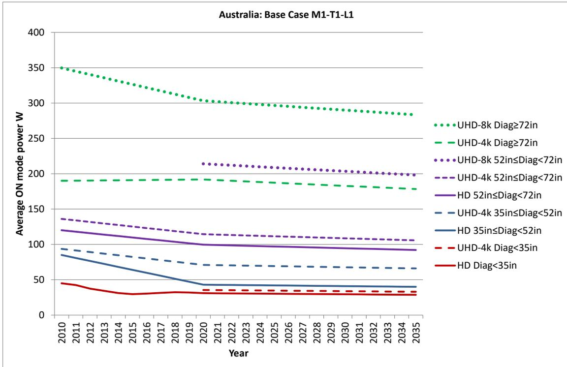
**Figure 13: Historical and projected on-mode power for televisions by size range and resolution, Australia. Sales weighted data to 2020, projections at -0.5% per annum to 2035. Average power within each size range will be increasing as the share of higher resolution models increases over time.**
