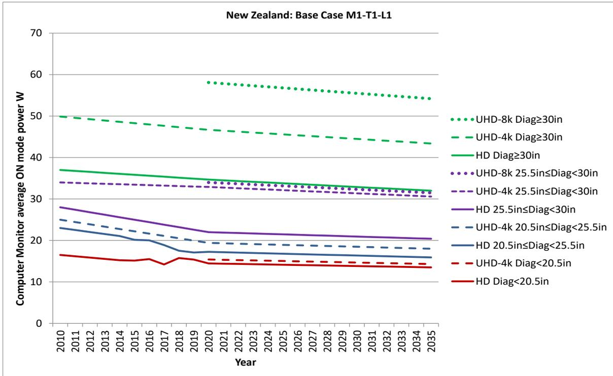
**Figure 32: Historical and projected base case on-mode power for computer monitors by size range and resolution, New Zealand**
