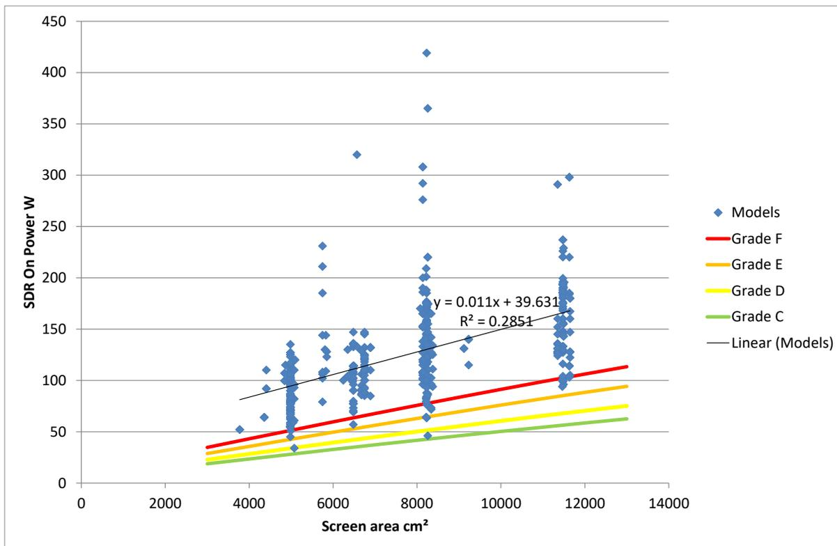
**Figure 40: Linear regression of screen area versus on power for European products within the EU regulation size scope**
