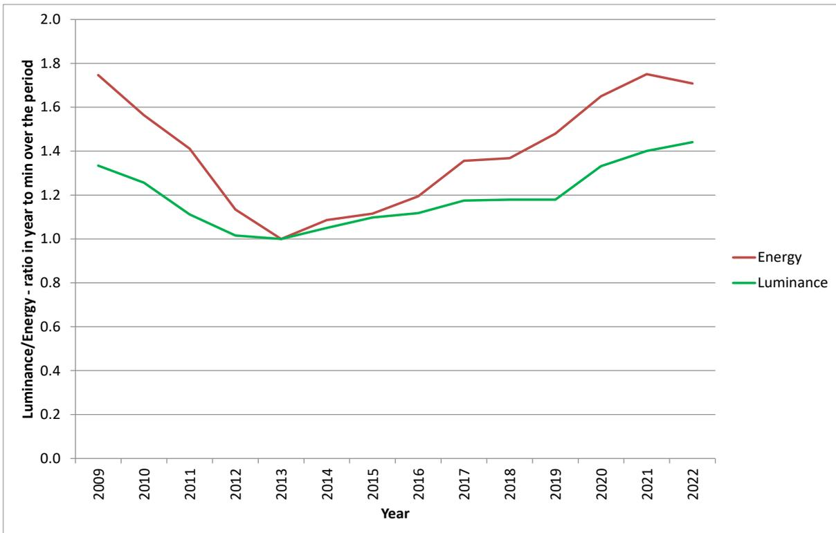
**Figure 48: Relative changes in energy and screen luminance for televisions over the period 2009 to 2022 (based on min).**
