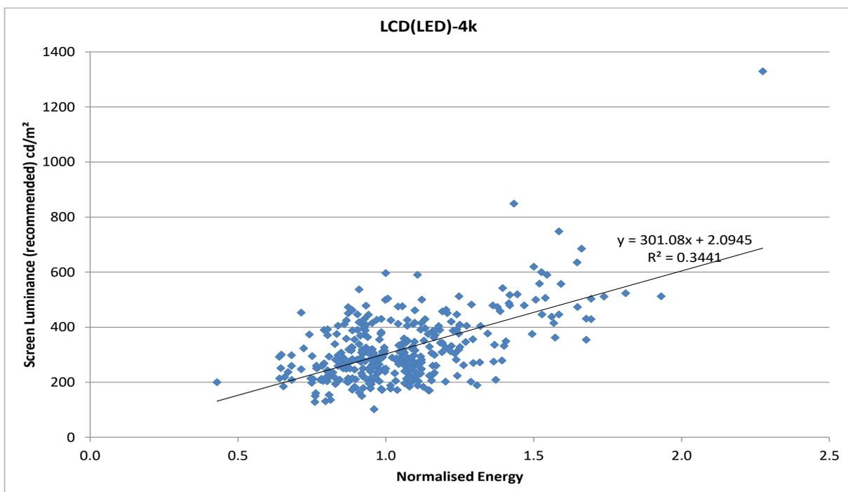
**Figure 53: Screen luminance as a function of normalised energy consumption for LCD (LED) 4k televisions.**
