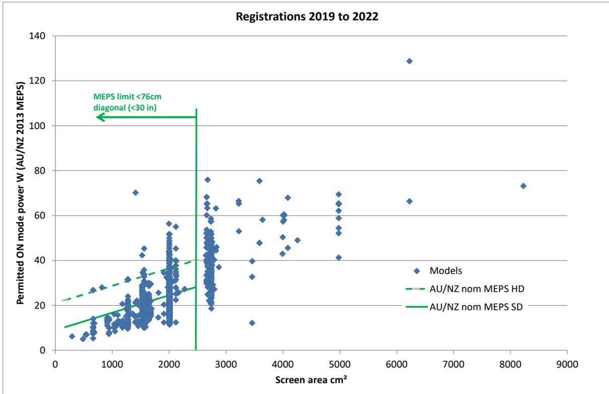
**Figure 29: Distribution of on-mode power showing MEPS levels for models registered 2019 to 2022**
