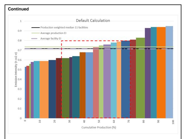
The graph shows emissions-intensity plotted by cumulative production for the example dataset. The proportion of production for the sector that contributes to the default value is indicated by the red dashed line. The emissions intensity default value is represented by the **black line** (0.717 tonnes  $CO_2$ -e/t production).
