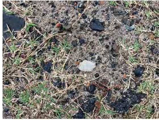
Photo 8. Close-up of asbestos containing material – sample FC-1
