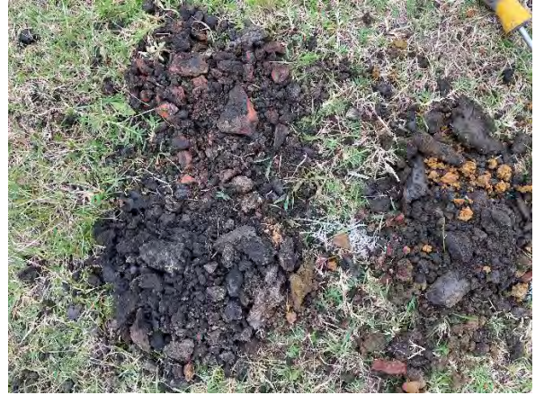
Photo 14. Fill material encountered at borehole BH1.
