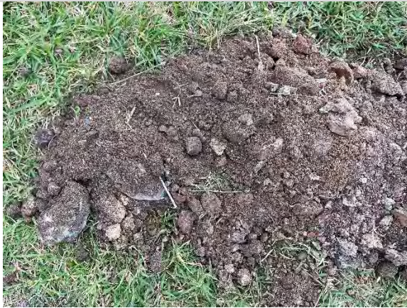
Photo 15. Deeper fill material encountered at borehole BH1
