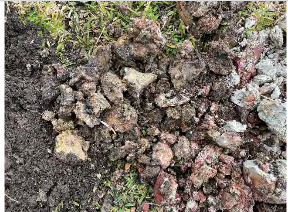
Photo 16. Natural residual soils encountered at borehole BH1.
