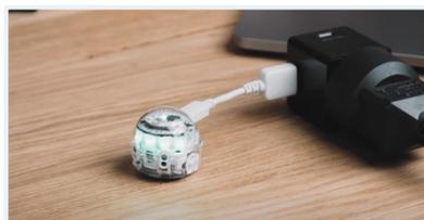
1 Plug Evo in to charge using an individual USB charging cable or charging base. Evo's LEDs will flash **green** while charging.
