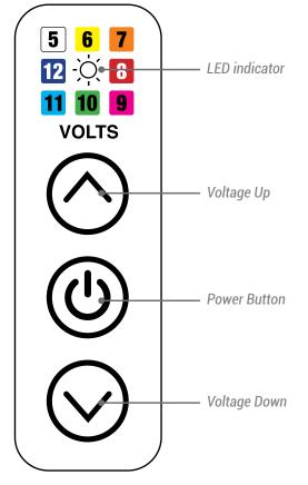
LED Indicator: Single blink = Whole Value Double blink = Half Increment Ex. Solid green indicates 10V Flashing green indicates 10.5V Battery Level Check: Press and hold power button until white. On release color = %
