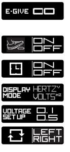
eGive: Use the up and down buttons to select level. Level 0 = disabled, Level 1 = Hard, Level 2 = Medium and Level 3 = Soft. When changing eGive please allow machine to finish sensing needle before using.
