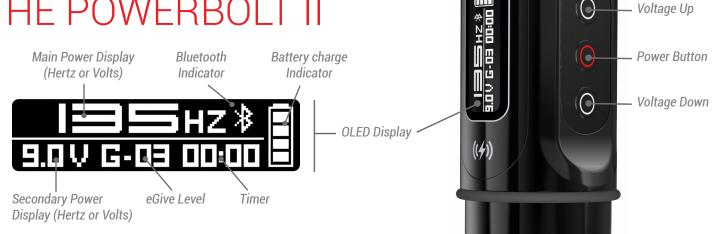
Battery Charge: 4 bars = 100%, 3 bars = 75%, 2 bars = 50% and 1 bar = 25%.
