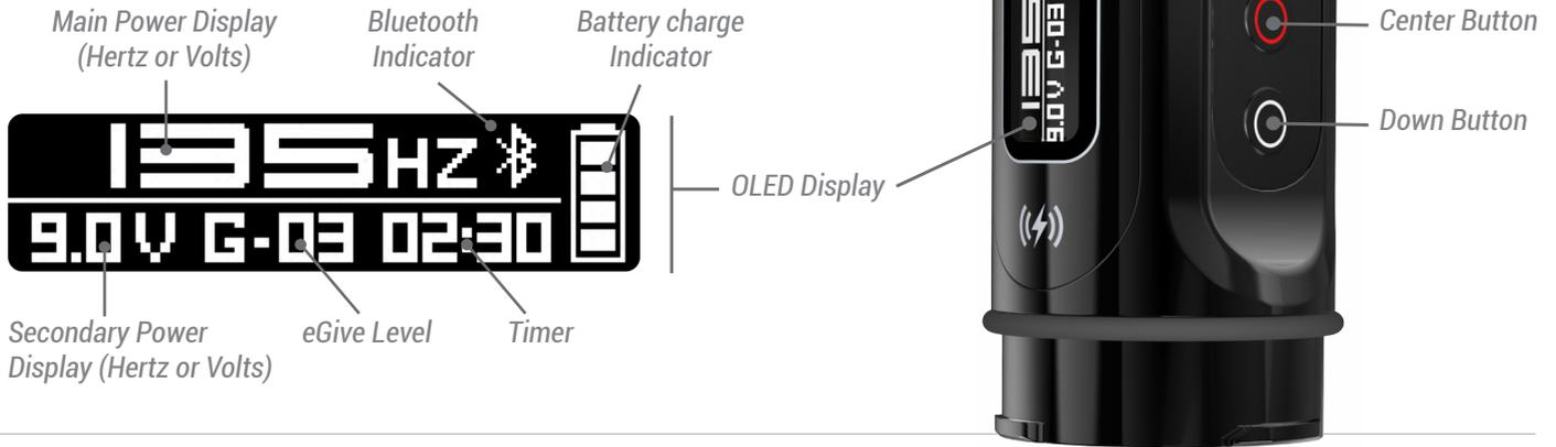
**Battery Charge:** 4 bars = 100%, 3 bars = 75%, 2 bars = 50% and 1 bar = 25%.
