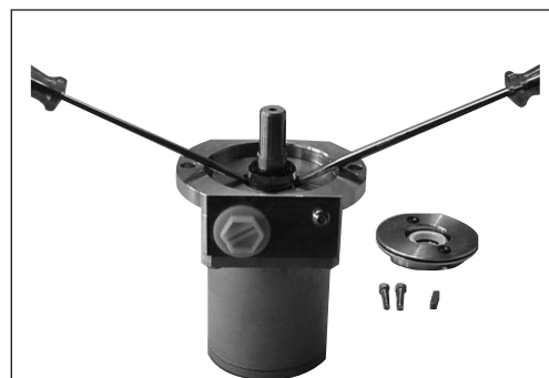
4. Remove the shaft seal using two screwdrivers. Caution: Avoid scratching the sealing surface on the shaft.
