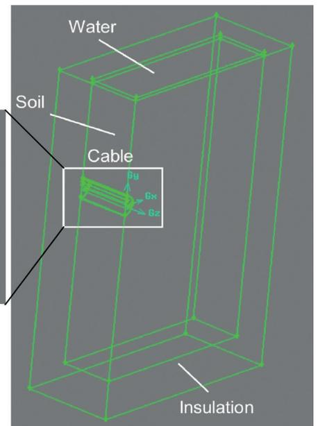
Figure 6: Experimental setup: Sketch
