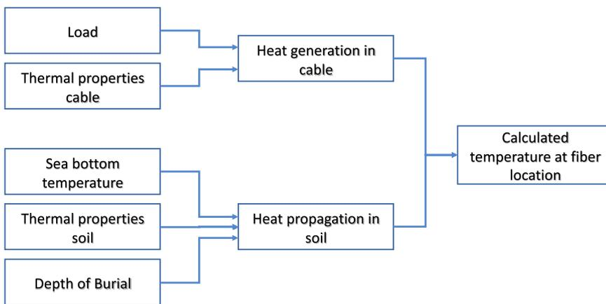
Figure 3: Block diagram of the Burial of Depth calculation model
