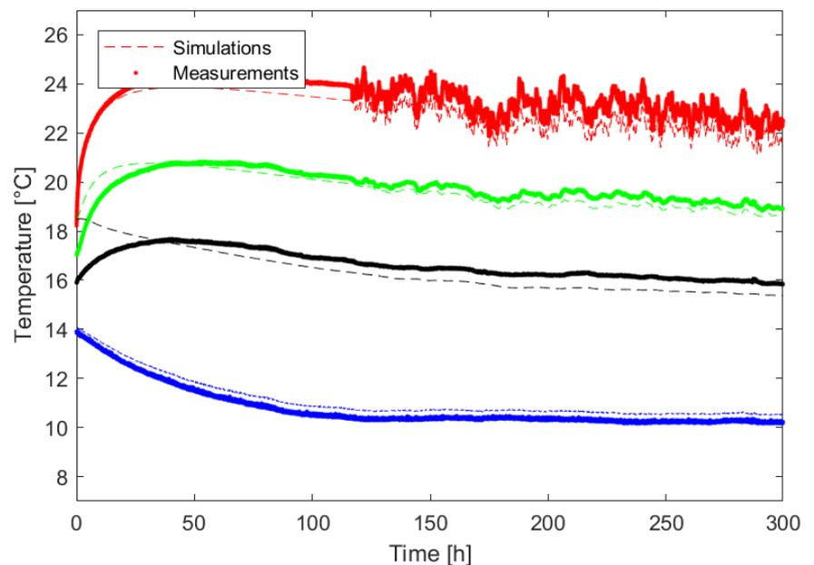
Figure 7: Comparison between experimental results and CFD calculations, first 120h with steady state heat signal, afterwards a periodic heat signal. (red: temperature at boundary cable-soil 60cm below the water surface, green: soil temperature 45 cm below the water surface, black: soil temperature 30 cm below the water surface, blue: temperature at the water surface)
