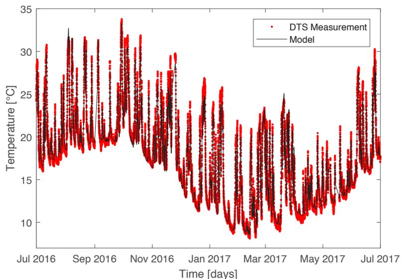
Figure 4: Comparison between measured Fibre temperature (red) and calculated fibre temperature (black)
