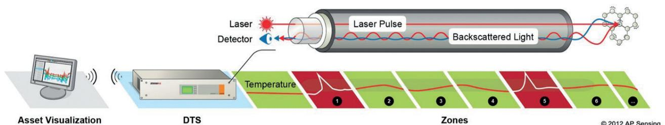
Figure 1: Schematic overview of the working principle of DTS (Source: AP Sensing)
