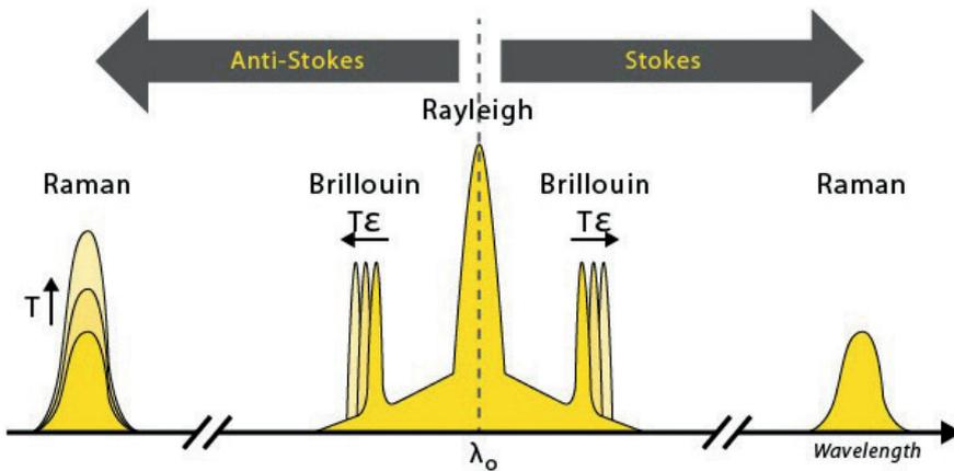
Figure 2: Wavelength of backscattered light (Source: Febus optics)
