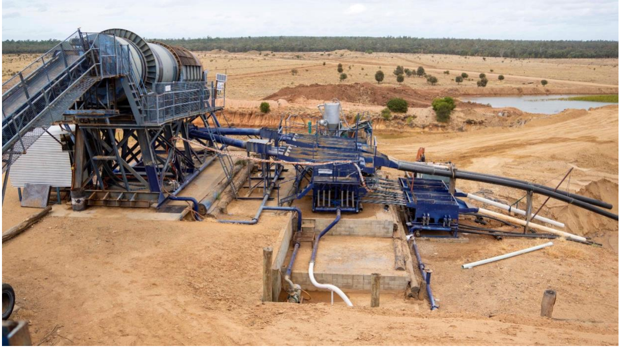
Figure 3. While the systems used in large-scale operations are similar to those run by a single person, the size sets them apart. Large washing plants can handle several metric tons of ore per hour and often run around the clock. This equipment requires a lot of water, so it is common to find manmade settling ponds nearby. Photo by V. Pardieu/GIA.
