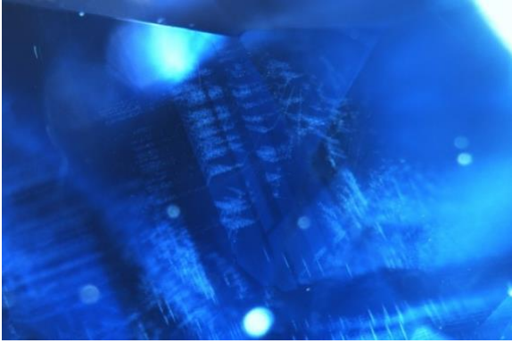
Figure 12. Flake inclusions in milky bands. Photomicrograph by Charuwan Khowpong; field of view 2.4 mm.
