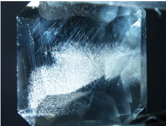
Figure 14. Rutile particles occur in various sizes and densities throughout this sapphire. Photomicrograph by Ungkhana Atikarnsakul; field of view 8.2 mm.
