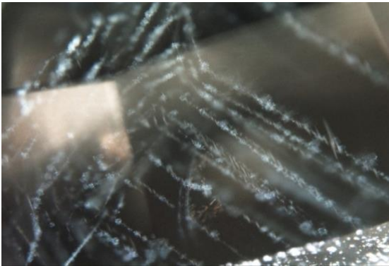
Figure 26. Strings of particles with short needles. Photomicrograph by Ungkhana Atikarnsakul; field of view 2 mm.
