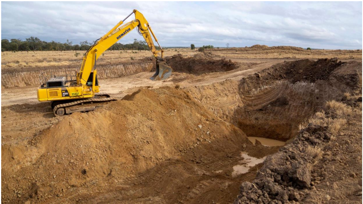
Figure 2. At large-scale operations, heavy equipment is used to expose the sapphire-bearing layers. Australia's strict mining practices require topsoil to be preserved, so this is dug out before the actual gem-rich layers are touched. Photo by V. Pardieu/GIA.
