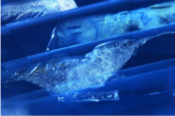
Figure 18. Several sapphires showed obvious twinning planes. In this case, they are associated with naturally healed fractures. Photomicrograph by Charuwan Khowpong; field of view 3.65 mm.
