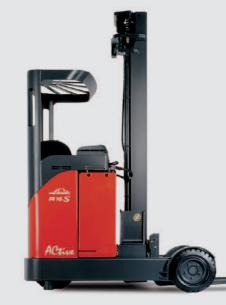
→ A short wheelbase, compact chassis dimensions and smooth electric power steering ensure easy and efficient manoeuvring
