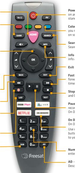
**Power** – turns the Box on and puts it into standby mode
