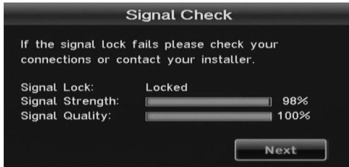
The signal check screen shows the strength and quality of the freesat signal received from your satellite dish. If the signal strength or quality is below 50%, you should check the satellite dish connection at the back of the receiver (switch the receiver off and reconnect the cable if necessary). If the connection is OK, consult your dealer or installer.
