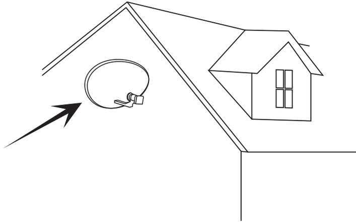
To receive freesat, you must connect your Plaza DS•100A receiver to an appropriate satellite dish, fixed in position and accurately pointed at the 28.2° East satellite position.
