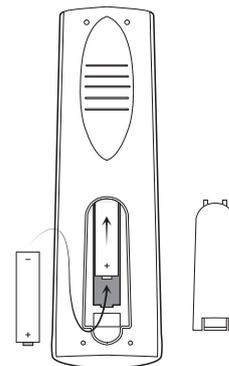
Take off the battery compartment cover from the back of the Plaza DS•100A remote control by lifting it up while pushing the catch. Insert the two AAA batteries supplied, as shown on the inside of the compartment, and replace the compartment cover.
