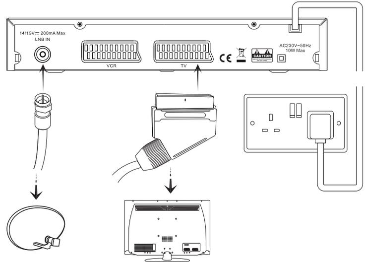
Connect the cable from your dish to the LNB IN socket at the back of the receiver (if the dish cable is fitted with a wall socket inside your home, you will need a connecting cable, which you can get from your installer).
