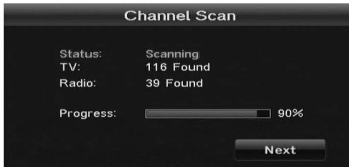
Your Plaza DS•100A receiver will take a couple of minutes to find and store the available freesat channels. The number of freesat TV and radio channels found is shown on the screen as the scan proceeds, along with an indication of how far the scan has to go. When the scan is complete, press the **OK** button to proceed.
