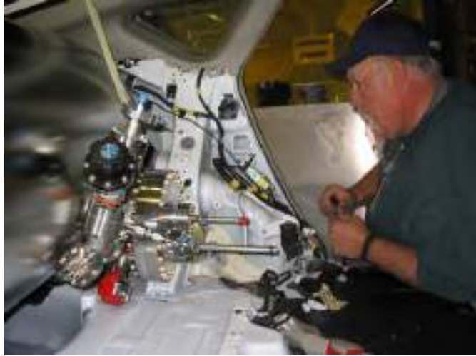
1. Install cryogenic capable pressure vessel in vehicle
