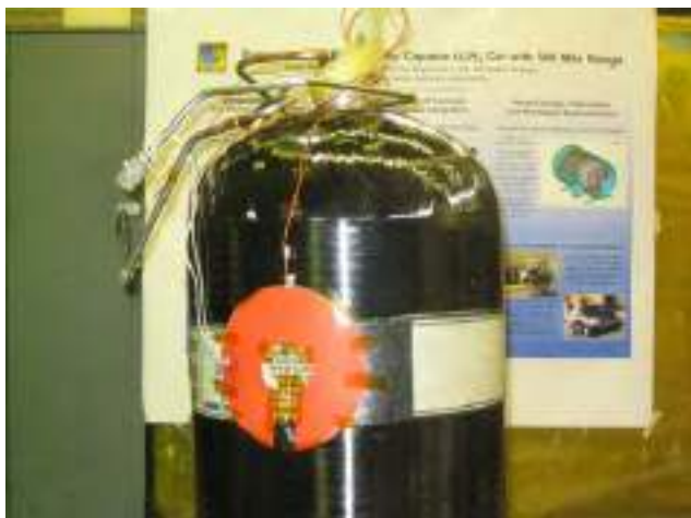
1. Attach instrumentation, heater and tubes to pressure vessel
