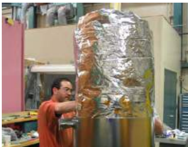
3. Slide insulated vessel into outer vacuum vessel
