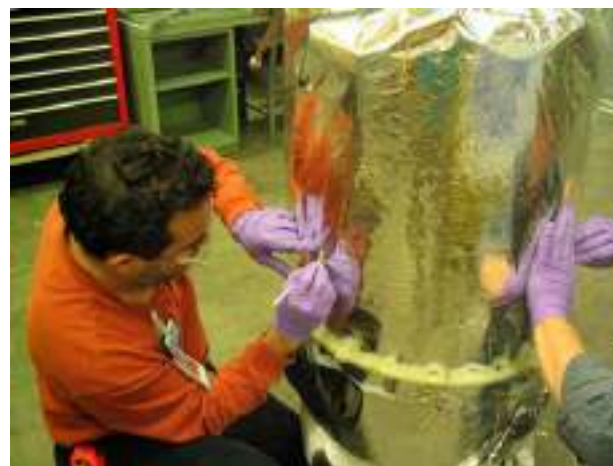
2. Install mechanical support rings and multilayer insulation
