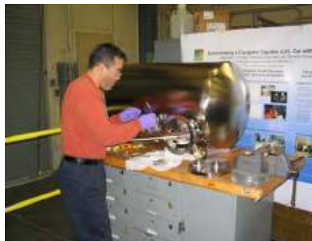
4. Weld vacuum vessel and install flanges for high pressure lines
