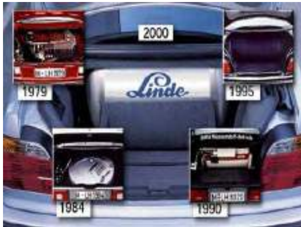
Liquid: thermal leak forces H 2 venting if parked ~2 days
